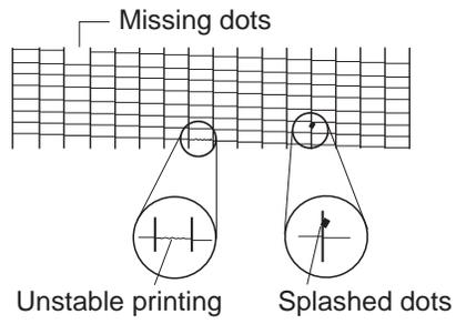
**Figure1-1 Defective Pattern Sample**
