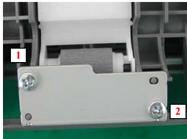
Figure 2-35. Reinstalling the ASF Frame Support Plate
