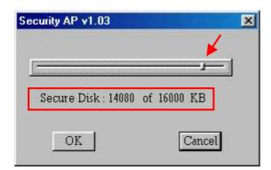
(3) Drag the bar to adjust the capacity of the "Protected" area.
