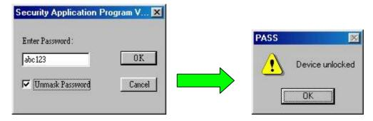
(2) When device is "unlocked", it will automatically switch to "Partition2" (the protected area)
