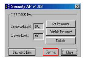
(1) Press "Format" to adjust the capacities of the SecurePenDrive.
