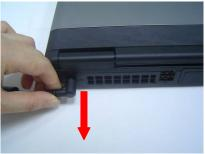
3. Turn the notebook over. Unlock and hold the latches, and remove the battery.
