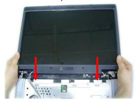
3. Secure 6 screws here, and then connect the Coaxial & inverter cable.
