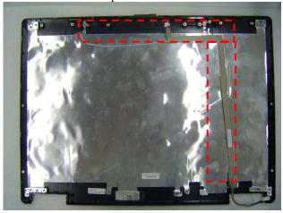
2. Install the wireless white wire module and secure 2 screws then paste 2 pieces of tapes to secure it.
