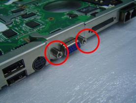
4. Secure 1 screw on the IO bracket to secure it.
