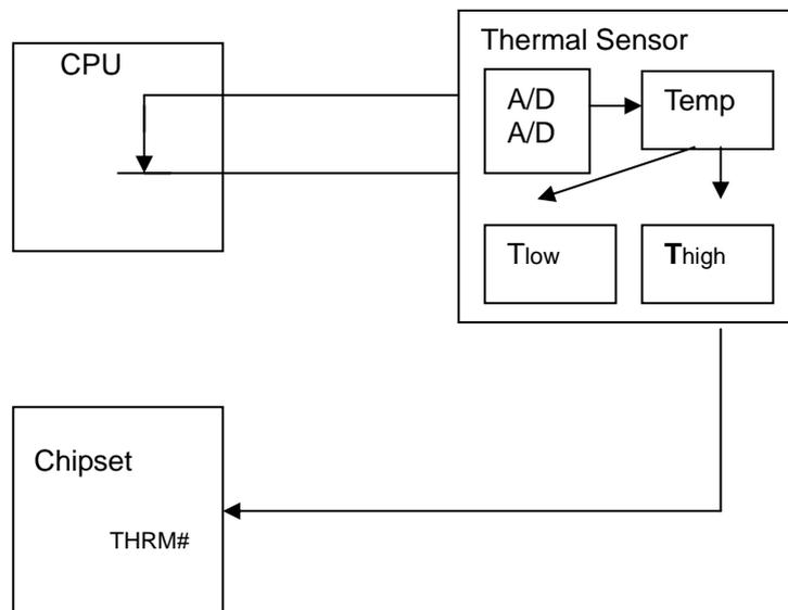
Thermal device function block diagram
