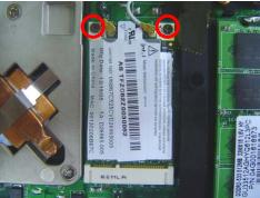
4. Connect the 2 antenna cables (black cable should be connected on main).
