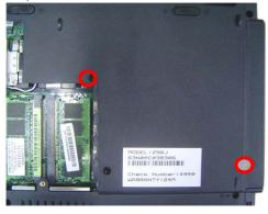
2. Put the CPU cover on and secure 3 screws (M2\*4L(K)) to fix it.
