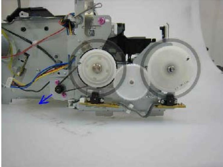
**Caution:** The red screws securing the paper feed motor may be loosened only at replacement of the paper feed motor unit. DO NOT loosen them in other cases.
