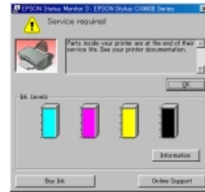
Figure 6-3. Maintenance error indication in STM3
