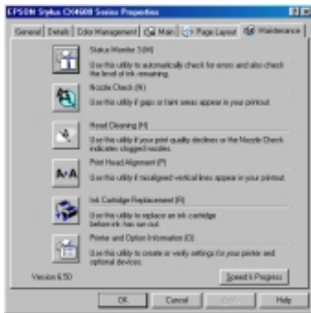
Figure 6-2. Head cleaning function in the printer driver utility
