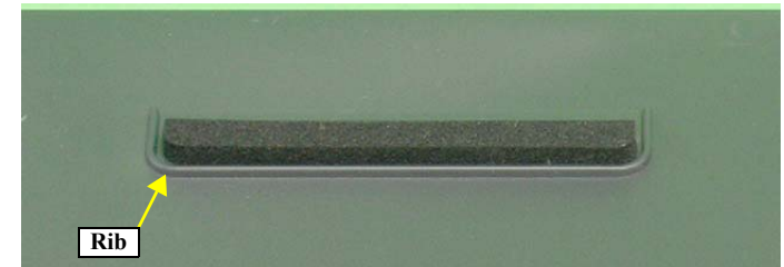
Figure 2-18. Reattaching the Stacker Paper Stoppers
