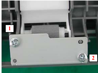
Figure 2-35. Reinstalling the ASF Frame Support Plate
