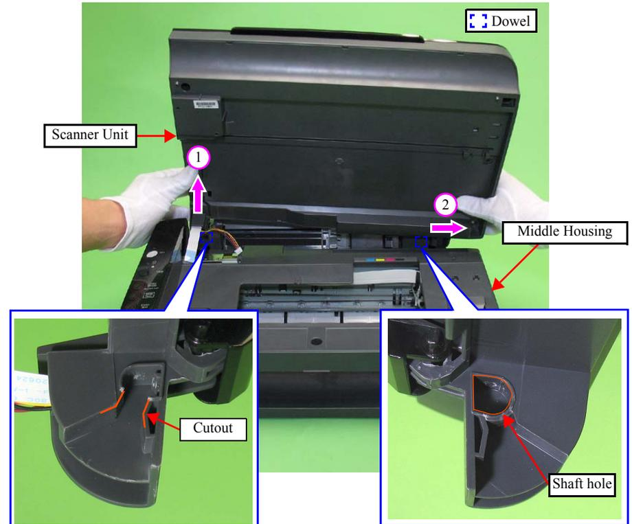
Figure 4-14. Removing the Scanner Unit (2)
