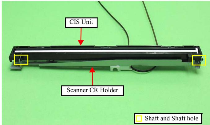
Figure 4-112. Removing the CIS Unit
