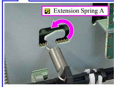
Figure 4-72. Removing the Main Frame (1)
