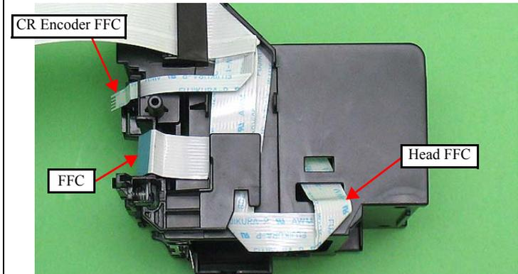
Figure 4-83. Installing the CR Unit (1)
