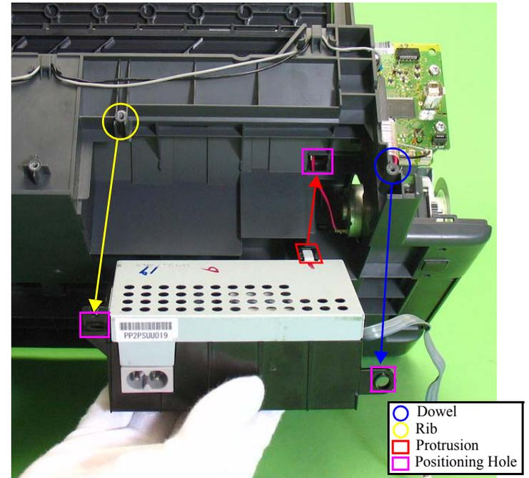
Figure 4-26. Installing the Power Supply Unit
