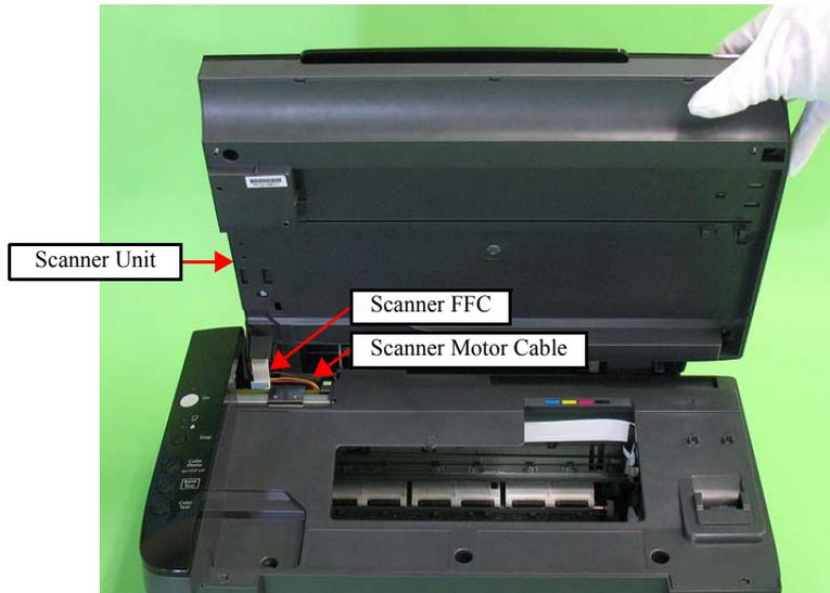
Figure 4-13. Removing the Scanner Unit (1)
