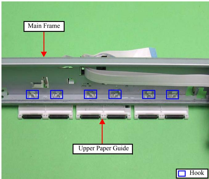
Figure 4-77. Removing the Upper Paper Guide
