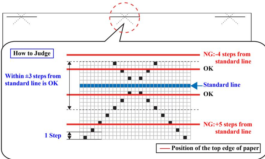
Figure 5-1. Top Margin Adjustment Printout Pattern
