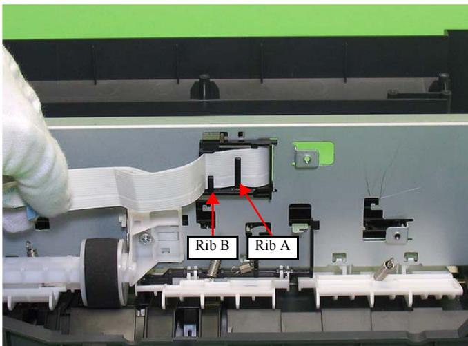
Figure 4-86. Installing the CR Unit (4)
