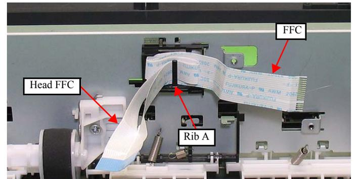
Figure 4-88. Installing the CR Unit (6)
