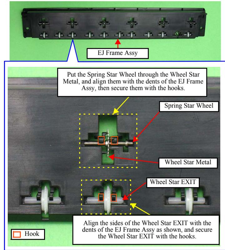
Figure 4-45. Assembling the EJ Frame Assy
