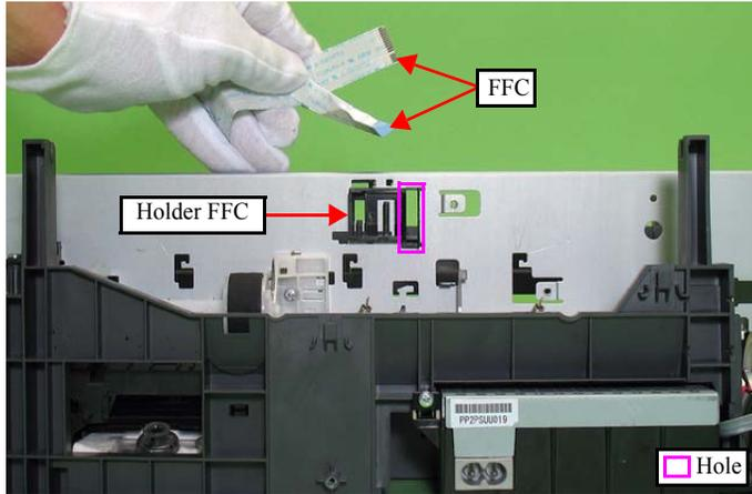
Figure 4-85. Installing the CR Unit (3)
