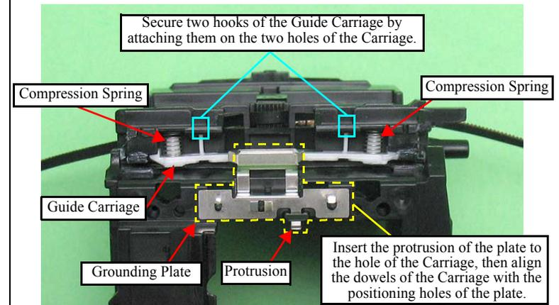
Figure 4-84. Installing the CR Unit (2)
