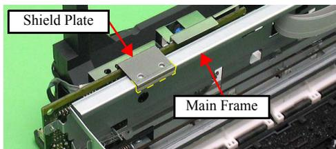
Figure 4-23. Installing the Main board
