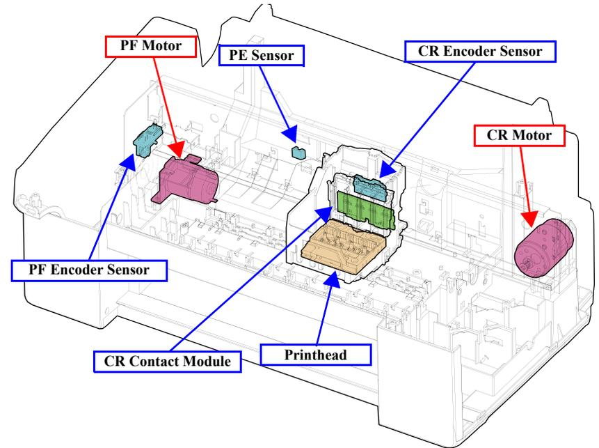
**Figure 2-2. Motors & Sensors in Printer Mechanism**
