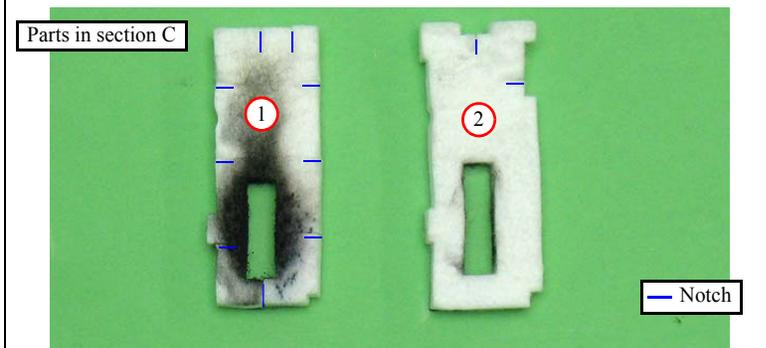
Figure 4-102. Installing the Waste Ink Pads (2)
