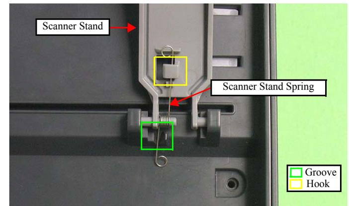
Figure 4-11. Installing the Scanner Stand
