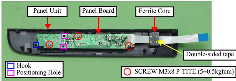
Figure 4-118. Removing the Panel Board
