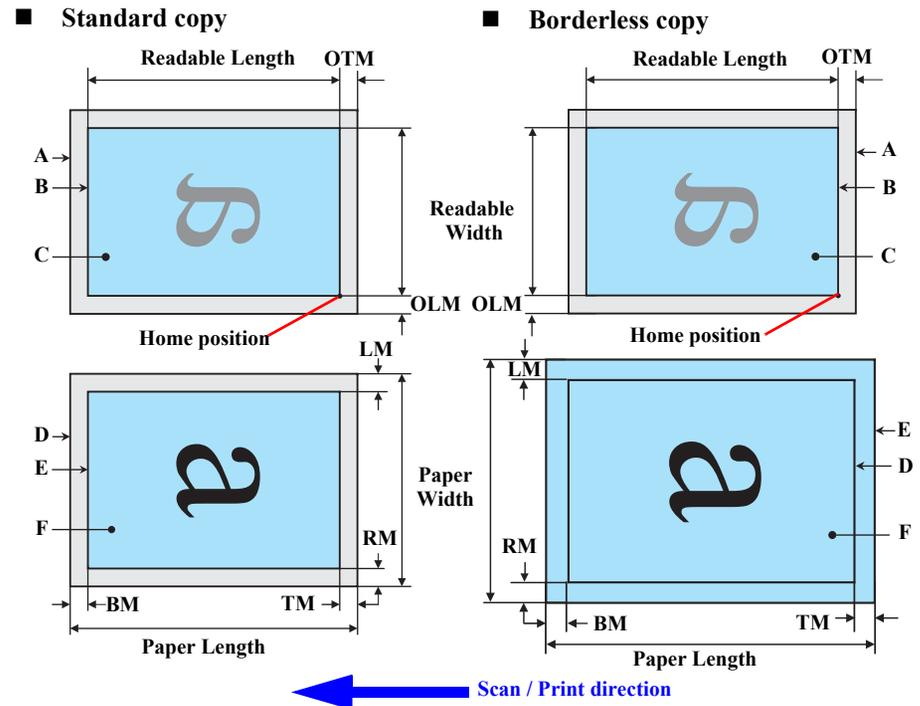
Figure 1-6. Relation Between Original and Copy (Borderless/With Borders)
