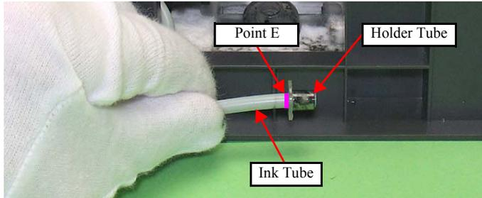
Figure 4-56. Installing the Pump Assy (1)
