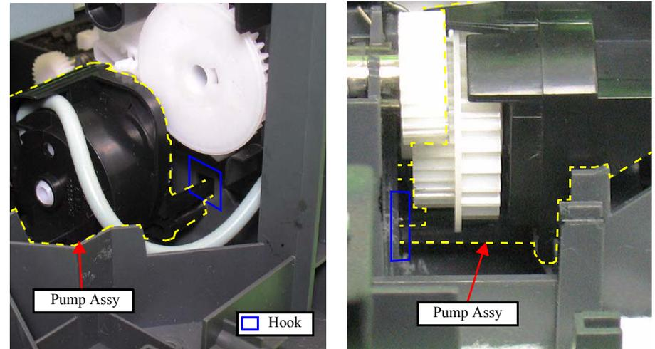
Figure 4-55. Removing the Pump Assy (2)
