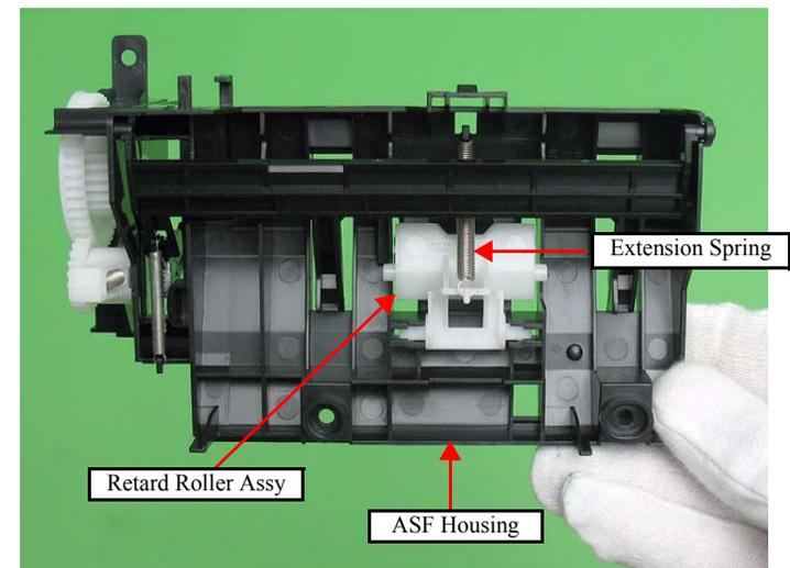
Figure 4-93. Removing the Retard Roller Assy
