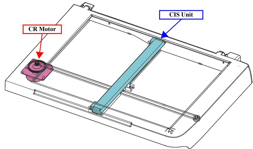
**Figure 2-3. CIS Unit and CR Motor in Scanner Mechanism**
