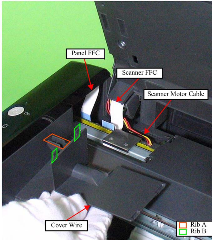
Figure 4-12. Installing the Cover Wire
