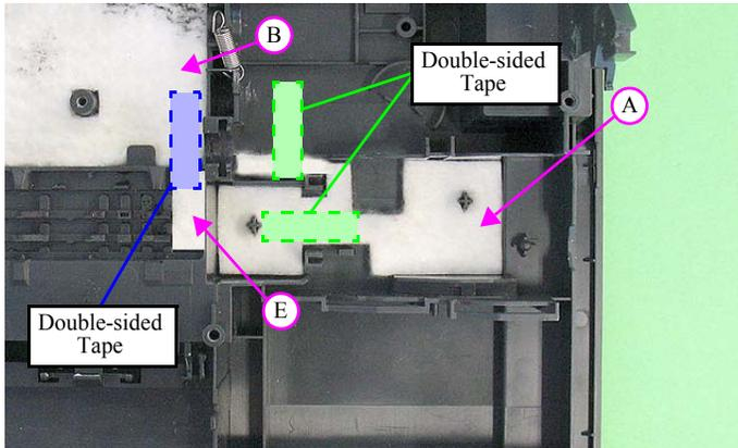
Figure 4-103. Installing the Waste Ink Pads (3)
