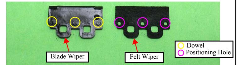
Figure 4-62. Assembling the Cap Assy (2)
