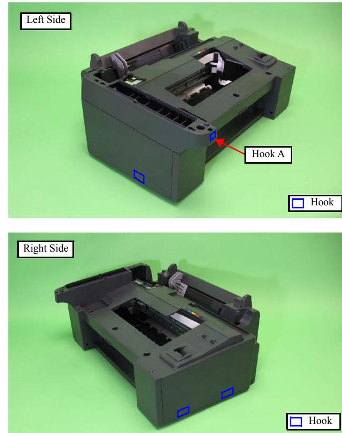
Figure 4-16. Removing the Middle Housing (2)
