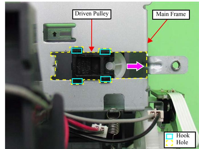
Figure 4-49. Installing the Driven Pulley
