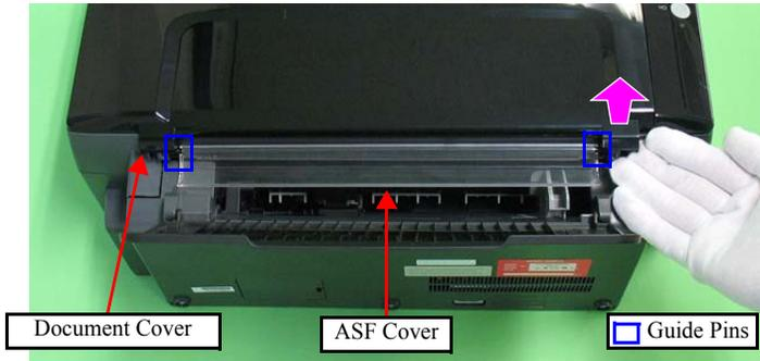
Figure 4-6. Removing the ASF Cover
