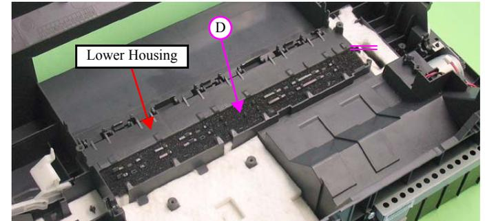
Figure 4-105. Installing the Waste Ink Pads (5)
