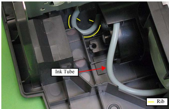
Figure 4-57. Installing the Pump Assy (2)
