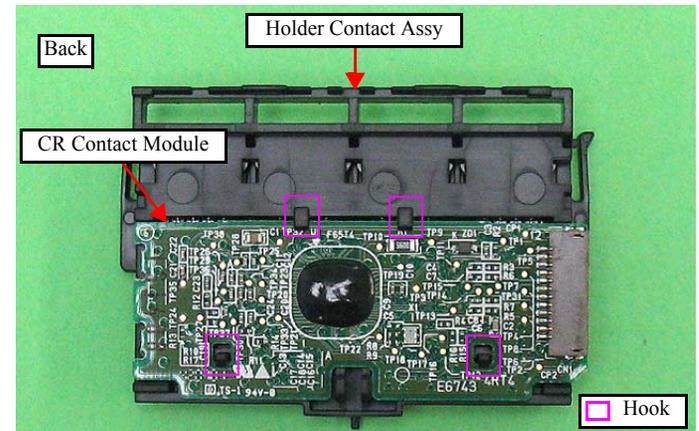
Figure 4-35. Assembling the Holder Contact Assy (2)
