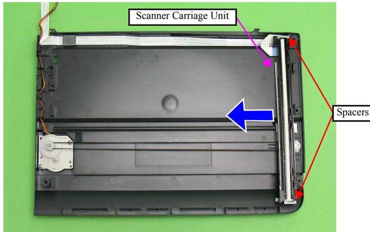
Figure 4-109. Moving the Scanner Carriage Unit
