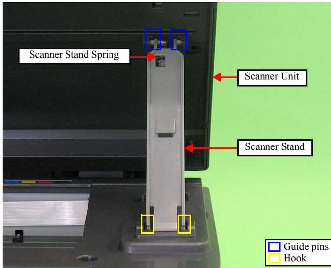
Figure 4-9. Removing the Scanner Stand
