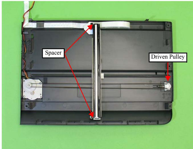
Figure 4-106. Installing the Spacer or the Driven Pulley
