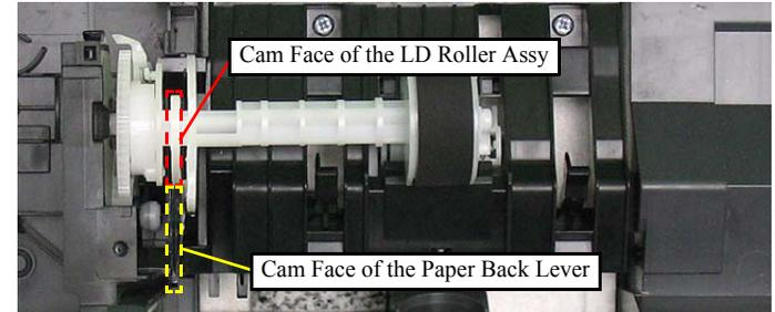
Figure 4-96. Installing the ASF Unit
