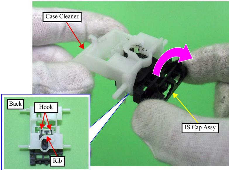
Figure 4-59. Disassembling the Cap Assy (2)
