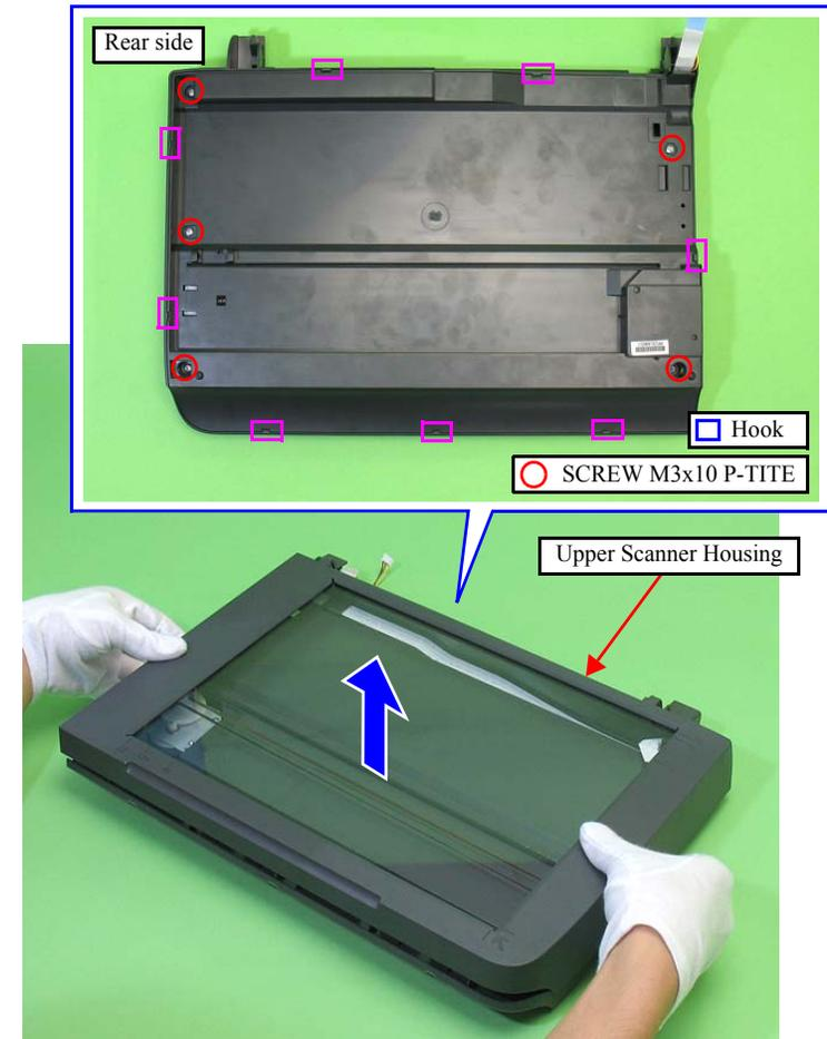
Figure 4-107. Removing the Upper Scanner Housing
