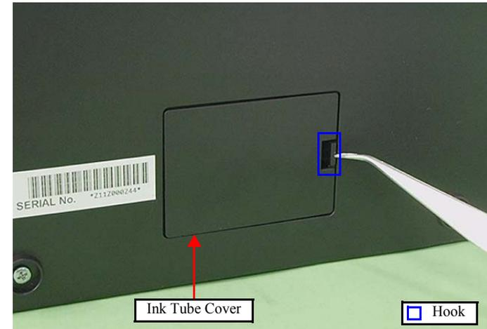
Figure 4-5. Removing the Ink Tube Cover
