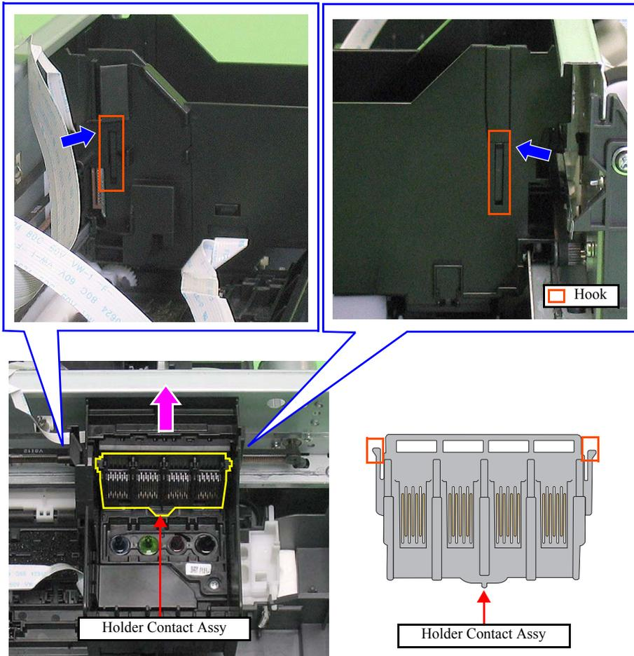
Figure 4-30. Removing the Printhead (4)
