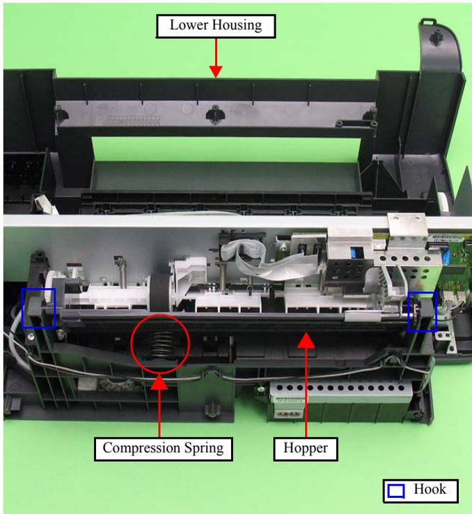
Figure 4-38. Removing the Hopper
