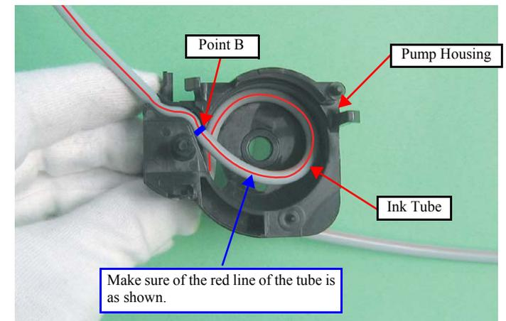
Figure 4-65. Assembling the Pump Assy (1)
