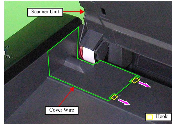
Figure 4-10. Removing the Cover Wire
