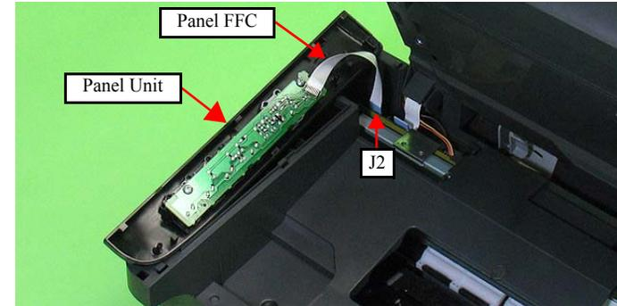
Figure 4-18. Removing the Panel Unit (2)
