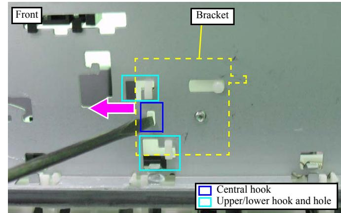
Figure 4-74. Removing the Main Frame (3)
