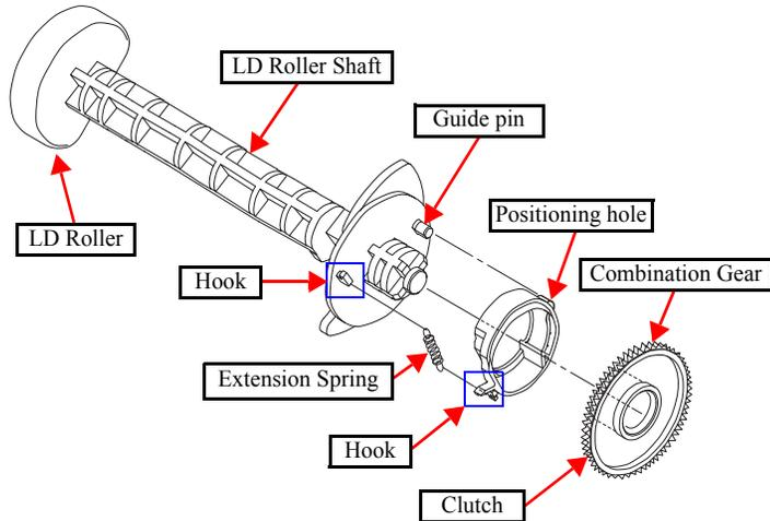
Figure 4-98. Assembling the LD Roller Assy (2)
