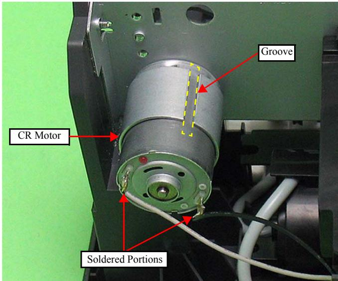
Figure 4-48. Installing the CR Motor
