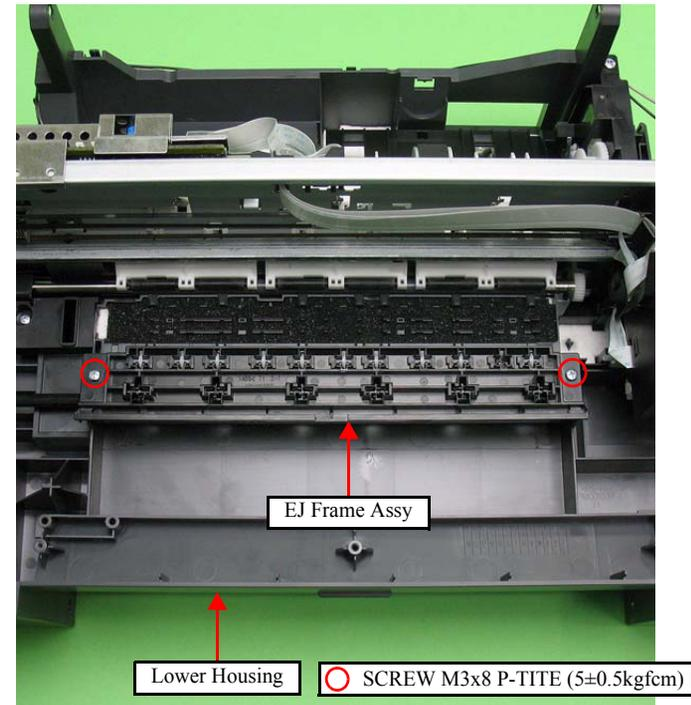
Figure 4-42. Removing the EJ Frame Assy
