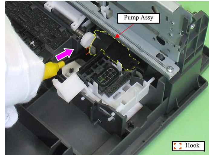
Figure 4-51. Removing the Cap Assy (2)
