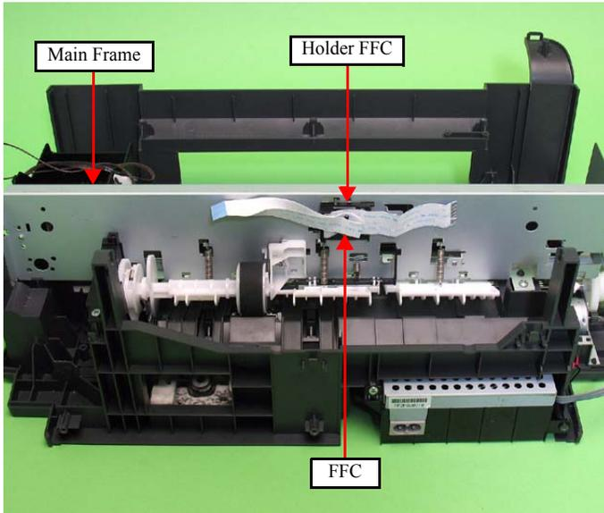
Figure 4-79. Removing the CR Unit (1)
