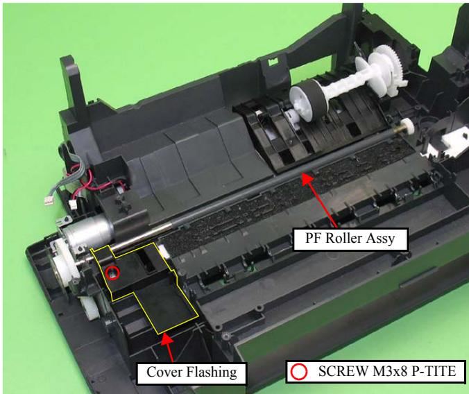
Figure 4-89. Removing the PF Roller Assy
