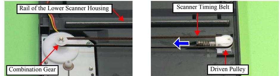
Figure 4-110. Removing the Scanner Carriage Unit (1)
