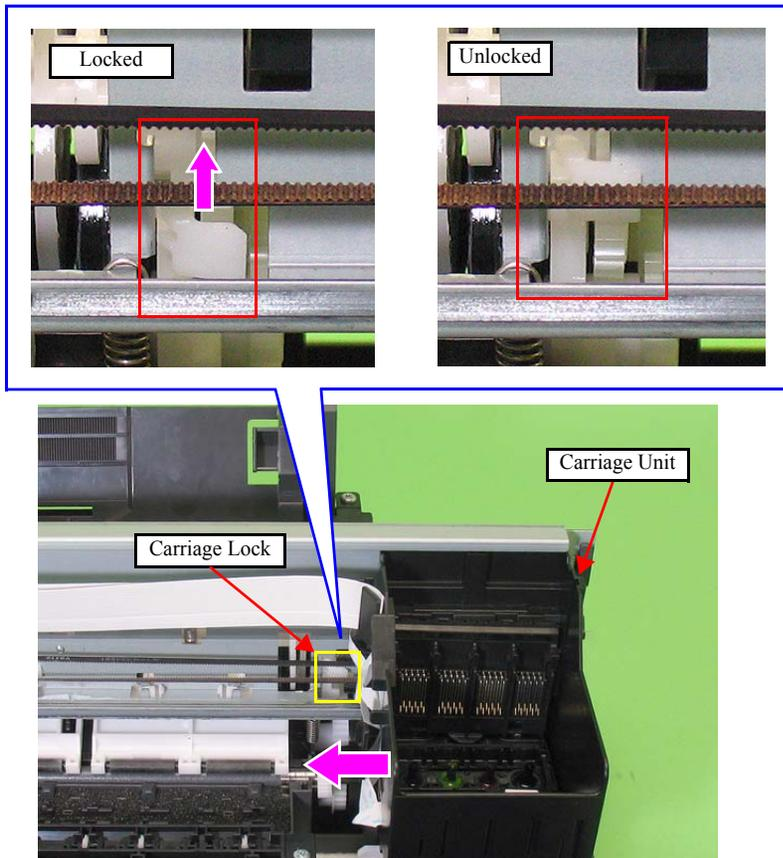
Figure 4-27. Removing the Printhead (1)
