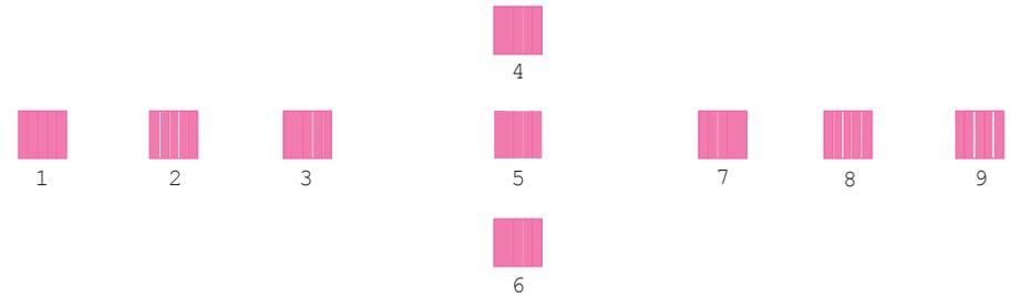
**Figure 5-3. Bi-D Adjustment Printout Pattern**
