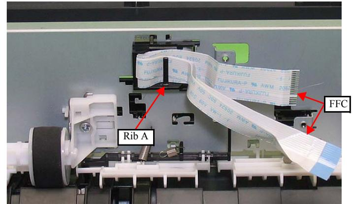
Figure 4-87. Installing the CR Unit (5)
