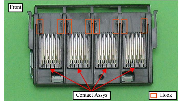
Figure 4-34. Assembling the Holder Contact Assy (1)
