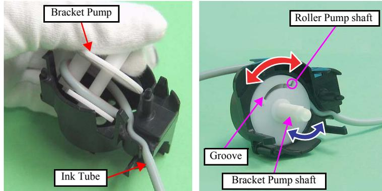
Figure 4-67. Assembling the Pump Assy (3)
