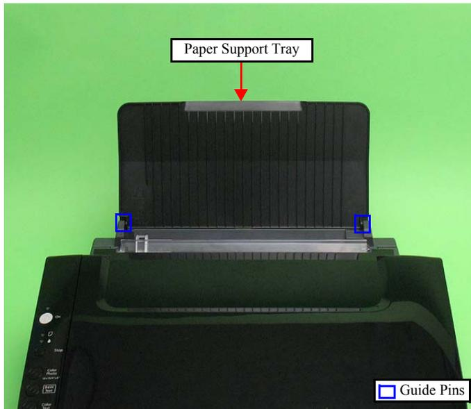
Figure 4-2. Removing the Paper Support Tray
