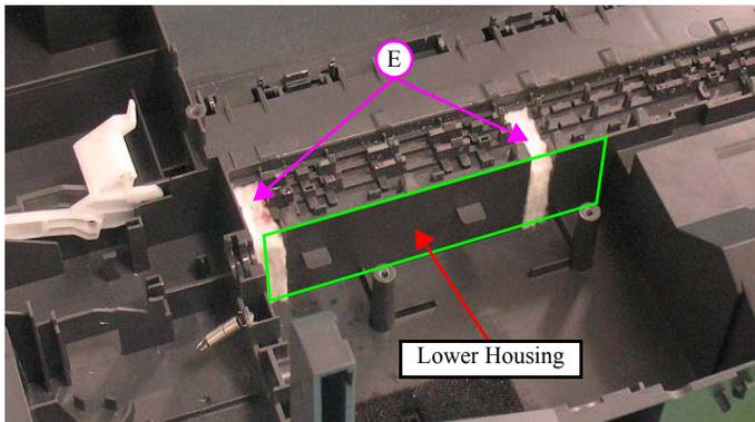
Figure 4-104. Installing the Waste Ink Pads (4)
