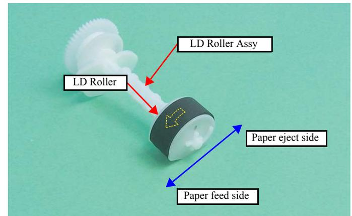
Figure 4-97. Assembling the LD Roller Assy (1)
