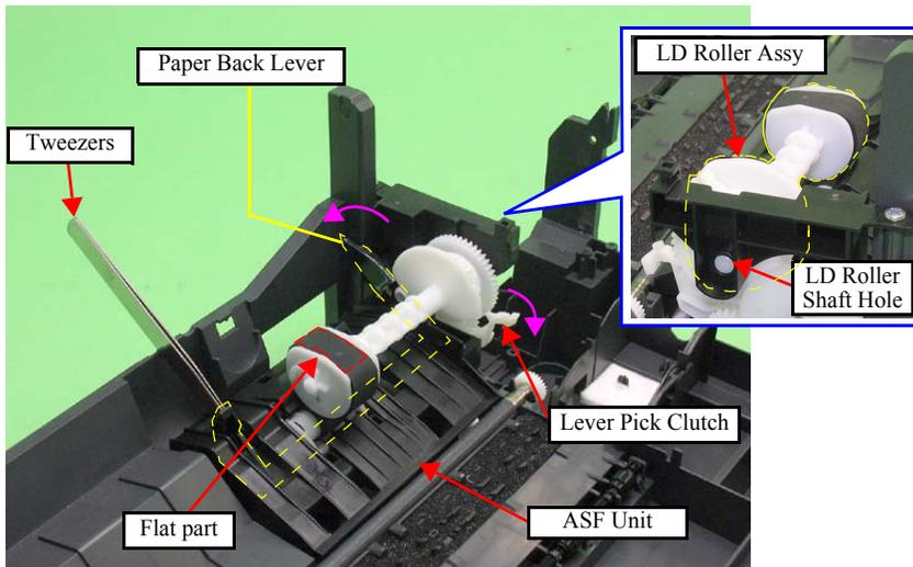
Figure 4-91. Removing the LD Roller Assy
