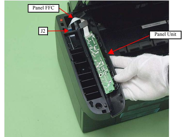
Figure 4-117. Removing the Panel Unit (2)
