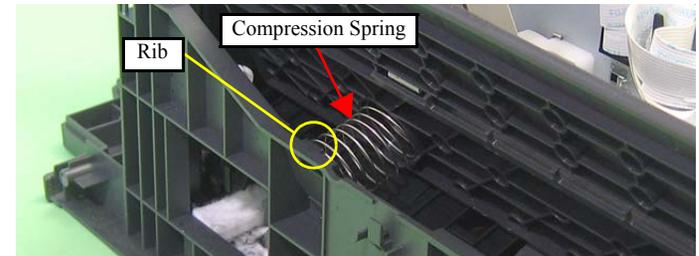
Figure 4-40. Assembling the Hopper
