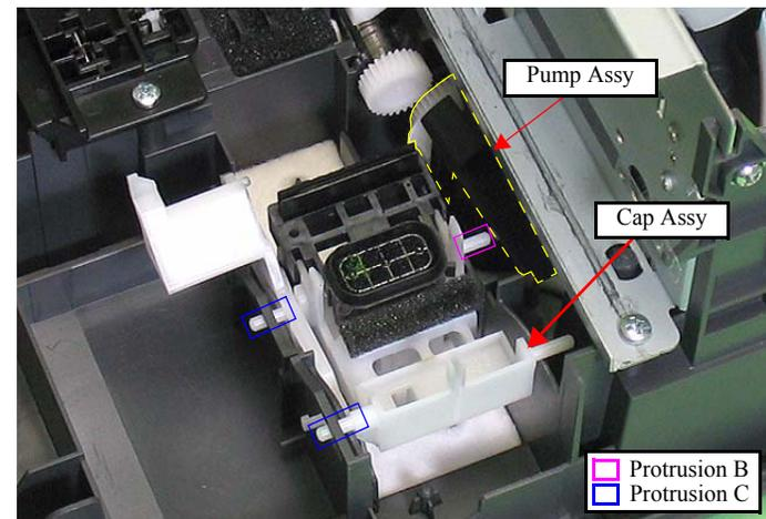
Figure 4-52. Removing the Cap Assy (3)
