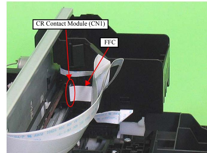
Figure 4-29. Removing the Printhead (3)
