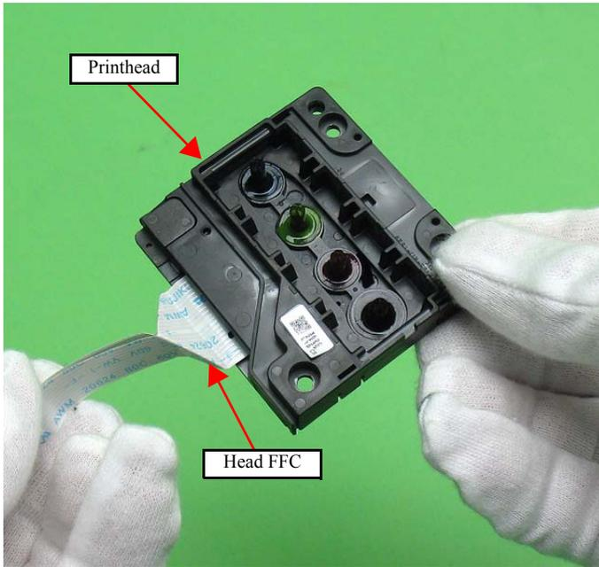
Figure 4-33. Removing the Printhead (7)
