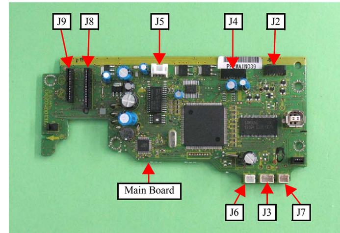
Figure 4-21. Removing the Main Board (1)
