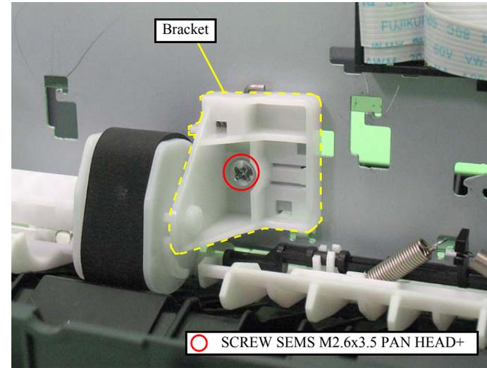
Figure 4-73. Removing the Main Frame (2)
