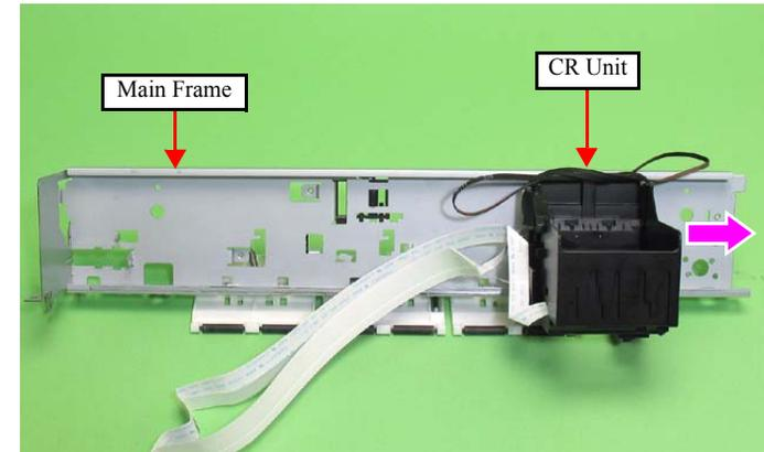
Figure 4-80. Removing the CR Unit (2)
