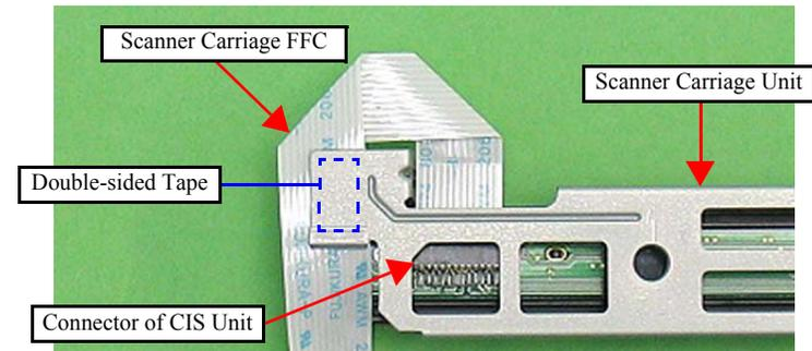
Figure 4-111. Removing the Scanner Carriage Unit (2)
