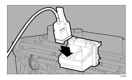
2. Lift the envelope sensor on the mechanism to raise the pivot to its maximum height.
