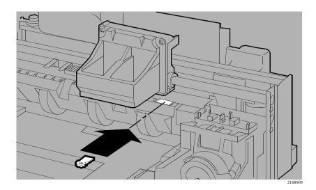
7. Lift the envelope sensor on the mechanism to raise the pivot to its maximum height. This will allow the pivot to release and capture the shim against the paper guide.
