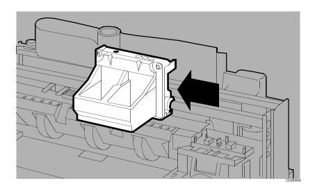
**2.** If removed, install the PPS Measure Tool. Snap the PPS Measure Tool into the cradle, just like installing a print cartridge.
