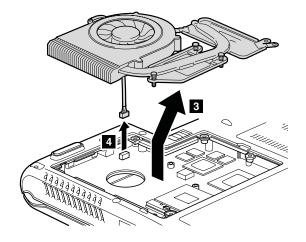
When installing: Make sure that the fan connector is attached firmly.
