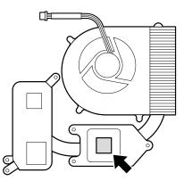
**When installing:** Before you attach a new heat sink assembly to the computer, peel off the covering film of thermal grease. Then attach the heat sink assembly to the computer.
