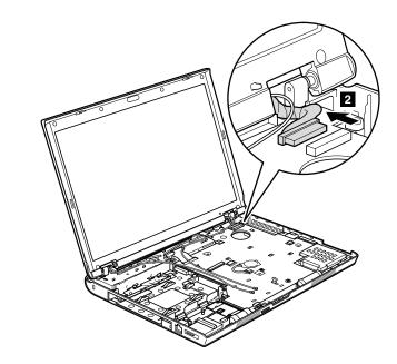
When installing: Make sure that the connector is attached firmly.
