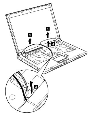
Pull out the wireless LAN antenna cables from the guide hole of the system board **3**, and release them from the cable guides of the frame **4**.
