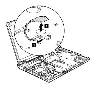
When installing: Make sure that the battery connector is attached firmly.
