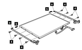
Remove the hinges ( a ) from the LCD panel.
