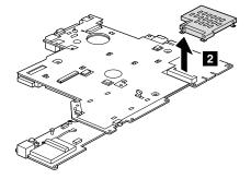
**When installing:** Make sure that the connector is attached firmly, and then fasten the screws.
