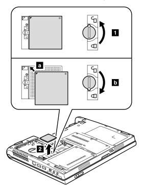
When installing: Place the CPU on the CPU socket **a**, and then rotate the head of the screw in the direction shown by arrow **b** to secure the CPU.
