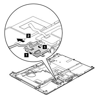
Slide the metal bracket of the fingerprint reader card in the direction shown by the arrow 3, and then remove the fingerprint reader card 4.
