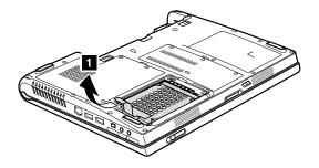
When installing: Make sure that the hard disk drive connector is attached firmly.
