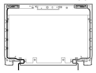
For the antennas with three cables
