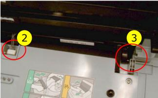
4. Loosen the screw in the red circle, separate the right side cover.
