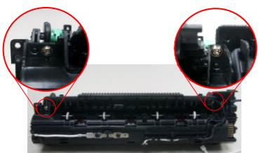
2. After Open FRAME-LOWER FUSER, Separate the GUIDE OUT FUSER.
