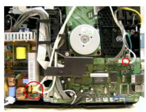
6. After loosen four screws in the red circle, pushing the holder shaft fuser to the right, and then separate the Fuser Ass'y from Printer.
