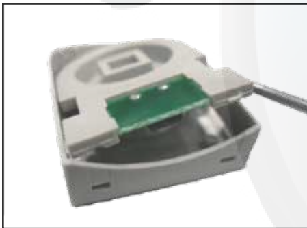
11. Carefully lift the chip from its housing.
