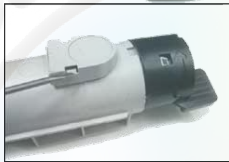
8. Using a small flathead screwdriver, press down on the tabs (shown on either side) to release the chip housing.
