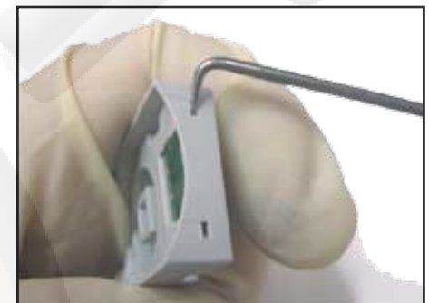
10. Unlock the actual chip from its housing by pressing the tabs (shown) using an angled hook tool.
