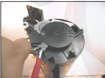
5. Take the Hopper Section and inspect the encoder wheel. It has probably been heat-welded against the plastic shaft requiring certain care during its removal. Insert a pair of long nose pliers to access the shaft at the center beneath the wheel and pry it off.
