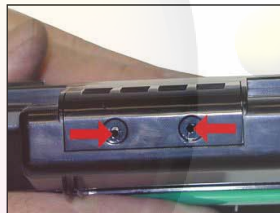
To replace the chip, drill out the two plastic rivets using a 5/64 bit and replace them with screws after the chip has been changed.
