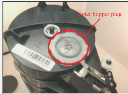
6. Remove the complete white fill plug at the side of the hopper. This is done by prying it open at the base near the border of the hole using a small flathead screwdriver. Opening the breather section (top portion of plug) does not give access to the hopper.
