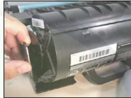
Open slightly one of the lateral edges to release the post engaging the toner hopper and the drum section together. Then repeat with the opposite side.
