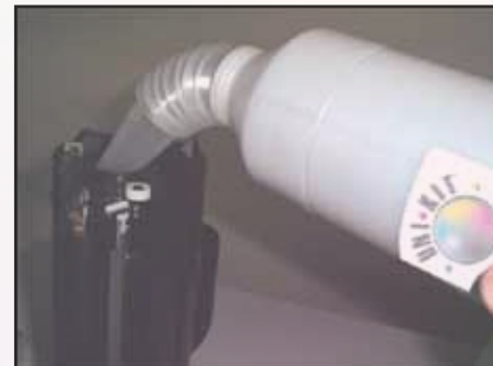
Refill the cartridge, once you are finished refilling, you may reassemble the cartridge.
