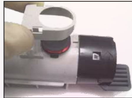
13. Place the housing over the chip as shown.
