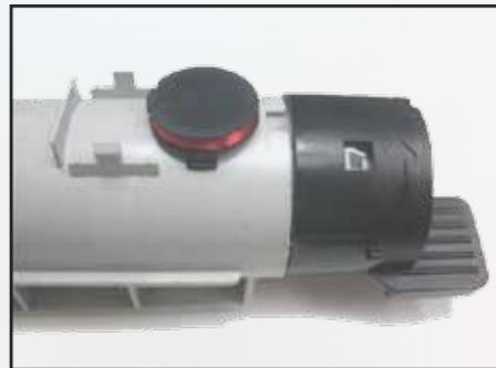
12. Place the new chip on the cartridge in the manner shown.
