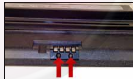
E.. Replace the chip by cutting the plastic rivets, drilling two holes, and setting two self tapping screws in place.
