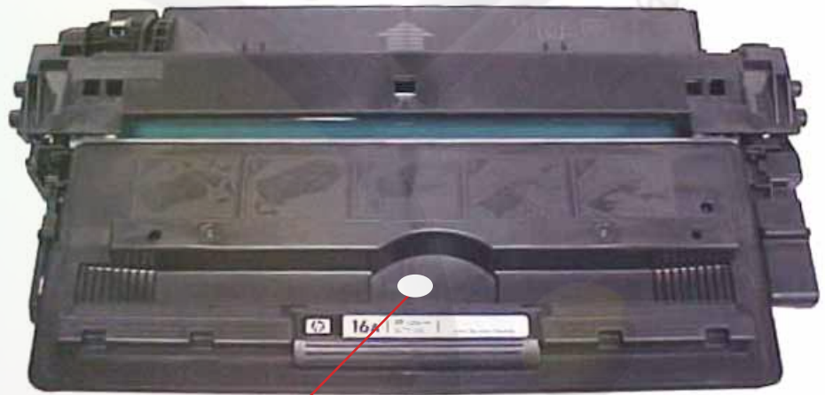
Create Refill Hole Here
