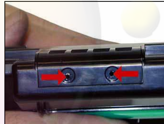
To replace the chip, drill out the two plastic rivets using a 5/64 bit and replace them with screws after the chip has been changed.
