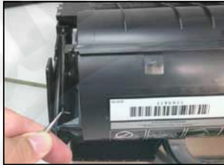
Disengage the two springs holding the sections together using a spring hook or small pointed pliers.
