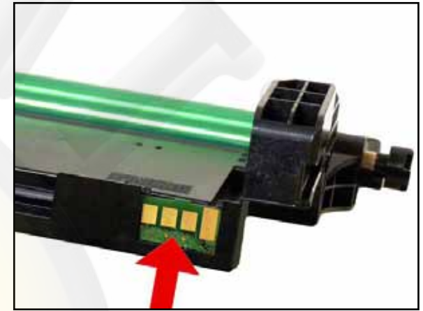
Remove the old chip, and replace it with the a new uni-kit replacement smart chip. After the chip is replaced, you may reverse the process to put the cartridge back together.
