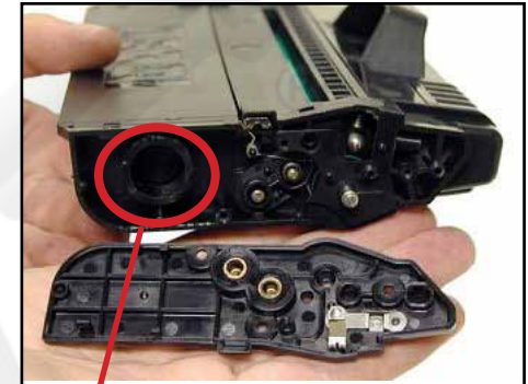
Carefully remove Toner Plug.
