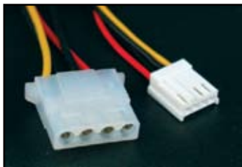
peripheral power connector (left) floppy power connector (right)
