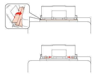
Load envelopes short edge first with the flap facing down and at the center of the rear MP tray.
