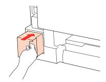
Push the button on either side of the rear unit at the same time, and then reattach the unit.
