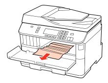
Close the front cover. If the jammed paper remains near the output tray, carefully remove the paper.
