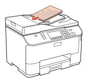
Slide the edge guide until it is flush with the originals.
