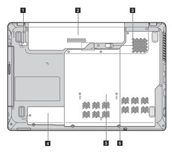
1 Battery latch - The manual battery latch is used to keep the battery pack secured in place.
