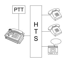
Connect the fax machine as the first device to the line and the home telephone system (HTS) like an additional device as second.
