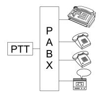
Connect the fax machine to an extension line of the private branch exchange (PABX). In order to operate your fax machine on an extension, you need to enter the appropriate settings in function 15.
